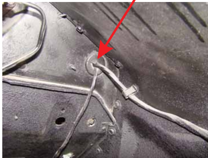
Front Light Wiring
